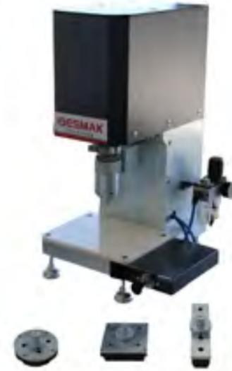
The pneumatic operated sample cutting Press test machine is easy to use and safe way to produce samples from materials such as plastics, fabrics, boards and paper. This machine operated up to 7 bar. Test sample cutters to any International standard.
