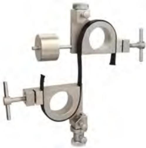
To test metal foils, ribbons, straps, etc. Manual and pneumatic modifications available.
