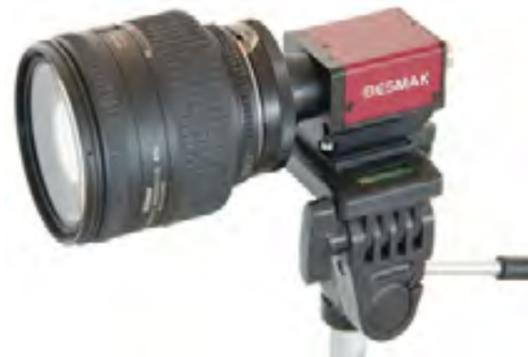
Video Extensometer is a contactless optical measurement system based on a digital camera and real time image processing. It measures the longitudinal and transverse strain between two applied lines with a rate of up to 4000 Hz. The strain data is transferred e.g. via an analogue signal or digital interface to the test machines for further processing or controlling.
