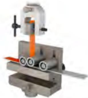
Peel grip, roller diameter 25 mm
